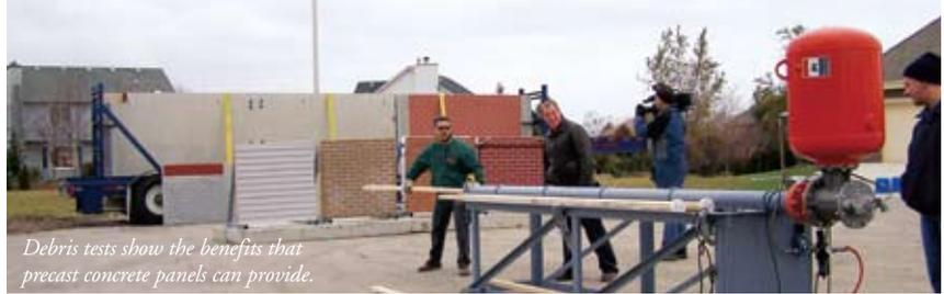
*Debris tests show the benefits that precast concrete panels can provide.*
