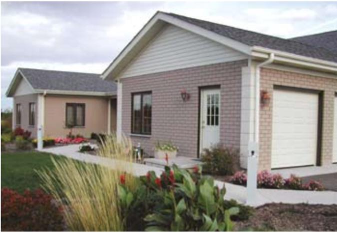
*Precast concrete panels can replicate the look of brick by using thin brick embedded in the panels or by creating a pattern on the face with formliners, as in this example from Prestress Engineering Corp.*
