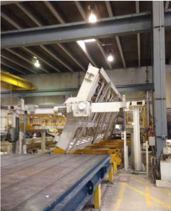
The first wythe of the insulated precast sandwich panel is turned upside down and then married to the second wythe using the innovative vacuum flipping table.
